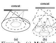
Figure 3: (a) Multi-scale grouping (MSG); (b) Multi-resolution grouping (MRG).
