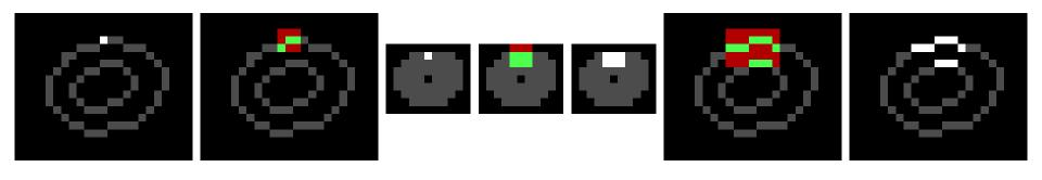
from left: (i) an active point is highlighted; a convolution with stride 2 sees the green active sites (ii) and produces output (iii), 'children' of highlighted active point from (i) are highlighted; a submanifold sparse convolution sees the green active sites (iv) and produces output (v); a deconvolution operation sees the green active sites (vi) and produces output (vii).
